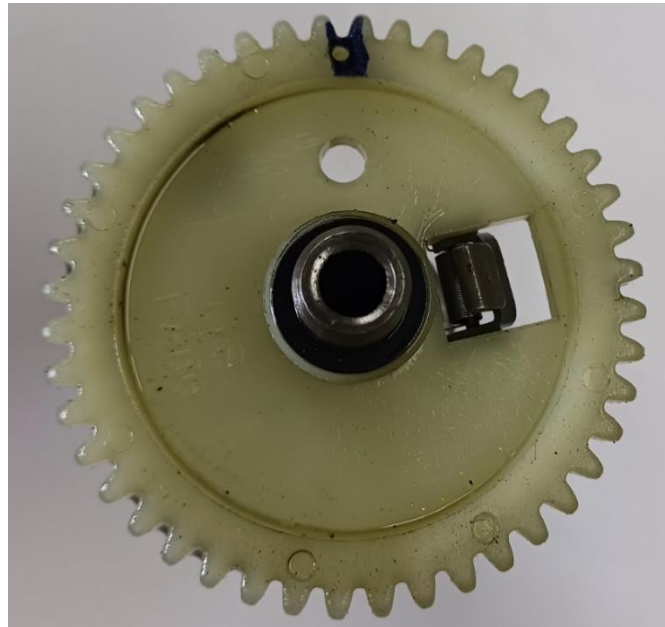
Camshaft Gear – 44 teeth
