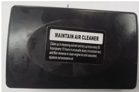
Airbox Front Cover (Part No: 152F-3)
