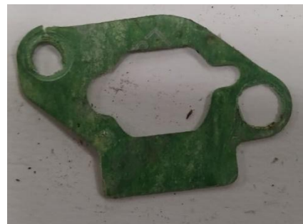
Airbox Gasket to Carburetor must be fitted.
