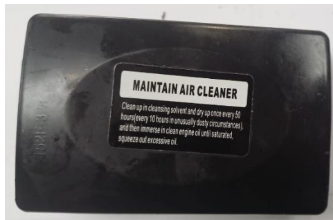
Airbox Front Cover (Part No: 152F-3)
