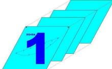
The inner plates should be contained within the confines of the endplates (as indicated by the dotted-line in diagram).
