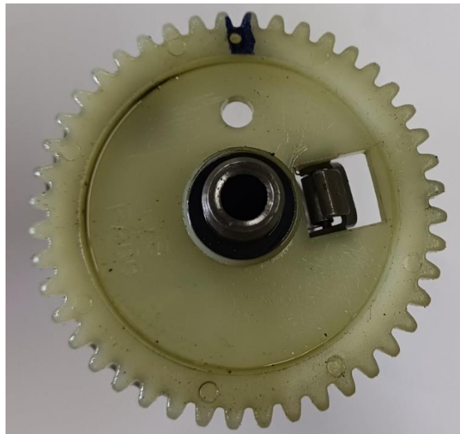
Camshaft Gear – 44 teeth
