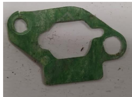
Airbox Gasket to Carburetor must be fitted.
