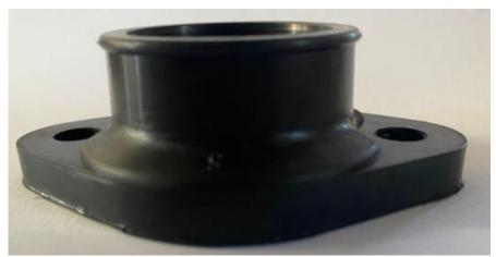
22.1.7 DDJ engine Exhaust Manifold: The only exhaust manifold permitted is as per the photos and dimensions below. No material may be added or removed. The exhaust manifold gasket as supplied must be fitted at all times:
