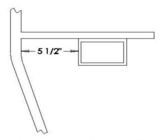
Note: The measurement for the battery box offset will be taken at the point closest to the crossmember, from the inside of the framerail to the ofside of the battery box.
