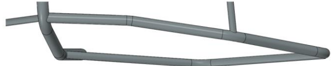
The central part of the members may be offset laterally to the outside (+Y) (vue de dessus / top view)
