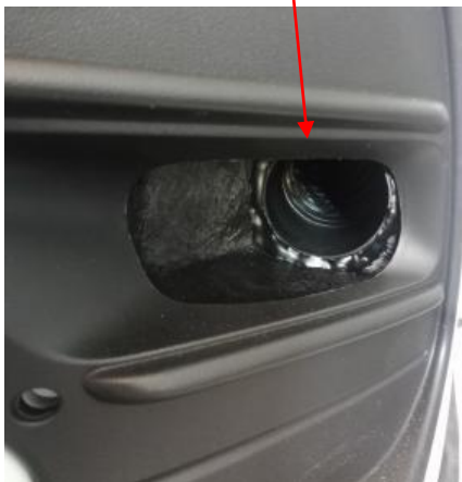
Facelift – Cars without gearbox cooler, may have the bumper insert without a hole fitted.
