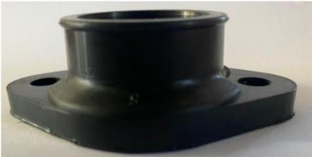
**i.** DDJ engine Exhaust Manifold: The only exhaust manifold permitted is as per photos and dimensions below. No material may be added or removed. The Exhaust Manifold gasket as supplied must be fitted at all times.
